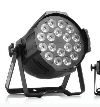
A high power LED Par in Aluminium housing with 18x10 W RGBW (4-in-1) LEDs. Equipped with DMX in/ out for daisy chaining multiple units together. It has preset programs that can be used in stand-alone mode. In the DMX settings there is the choice of a few channel modes with preset colours. The Aluminium housing and double stand make the fixture ideal for rental features, being lightweight and easy to setup.
