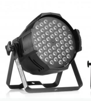
A high power LED Par in Aluminium housing with 54x3 W LEDs. Equipped with DMX in/out for daisy chaining multiple units together. It has preset programs that can be used in stand-alone mode. In the DMX settings there is the choice of a few channel modes with preset colours. The Aluminium housing and double stand make the fixture ideal for rental features, being lightweight and easy to setup.
