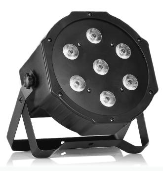
A high power LED Par in Plastic housing with 7x1 W LEDs. Equipped with DMX in/out for daisy chaining multiple units together. It has preset programs that can be used in stand-alone mode. In the DMX settings there is the choice of a few channel modes with preset colours. The plastic housing and double stand make the fixture ideal for rental features, being lightweight and easy to setup.
