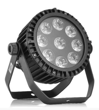
A high power LED Par in Aluminium housing with 9x8 W LEDs. Equipped with DMX in/out for daisy chaining multiple units together. It has preset programs that can be used in stand-alone mode. In the DMX settings there is the choice of a few channel modes with preset colours. The Aluminium housing and double stand make the fixture ideal for rental features, being lightweight and easy to setup.
