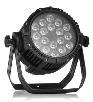
A high power LED Par in Aluminium housing with 18x12 W (6-in-1) LEDs. Equipped with DMX in/out for daisy chaining multiple units together. It has preset programs that can be used in stand-alone mode. In the DMX settings there is the choice of a few channel modes with preset colours. The Aluminium housing and double stand make the fixture ideal for rental features, being lightweight and easy to setup.
