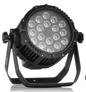
A high power LED Par in Aluminium housing with 18x12 W (6-in-1) LEDs. Equipped with DMX in/out for daisy chaining multiple units together. It has preset programs that can be used in stand-alone mode. In the DMX settings there is the choice of a few channel modes with preset colours. The Aluminium housing and double stand make the fixture ideal for rental features, being lightweight and easy to setup.
